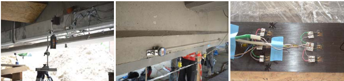
Figure 12. Vertical deflections, concrete and CFRP strain measured during strengthening
