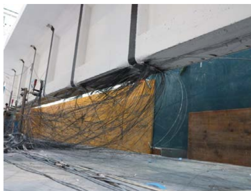
Figure 6: Failure mode of the strengthened girder (left) and measurements of deflection in the reference and the strengthened girder (right) [4]
